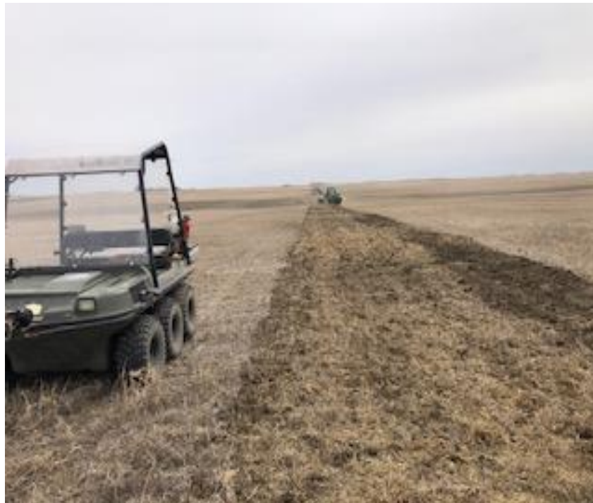
Side by side used to check ahead of tractor for soft spots to avoid if needed
